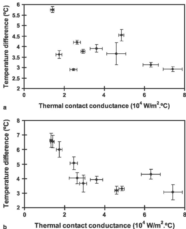
Fig. 8. Temperature difference in computer testing versus thermal contact conductance in guarded hot plate measurement: (a) computer A and (b) computer B.
