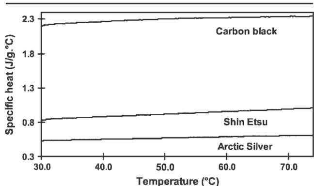
Fig. 5. Variation of the specific heat with temperature for each of three thermal pastes.
