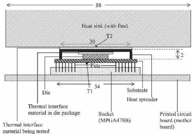
Fig. 2. Experimental setup using computer B for application-oriented testing of various thermal interface materials. T1 and T2 are thermocouples. All dimensions are in millimeters.
