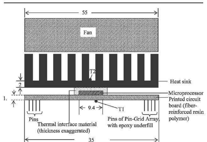
Fig. 1. Experimental setup using computer A for application-oriented testing of various thermal interface materials. T1 and T2 are thermocouples. All dimensions are in millimeters.
