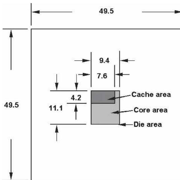
Fig. 3. Functional die layout for computer A. All dimensions are in millimeters and were taken from a photograph of the die.
