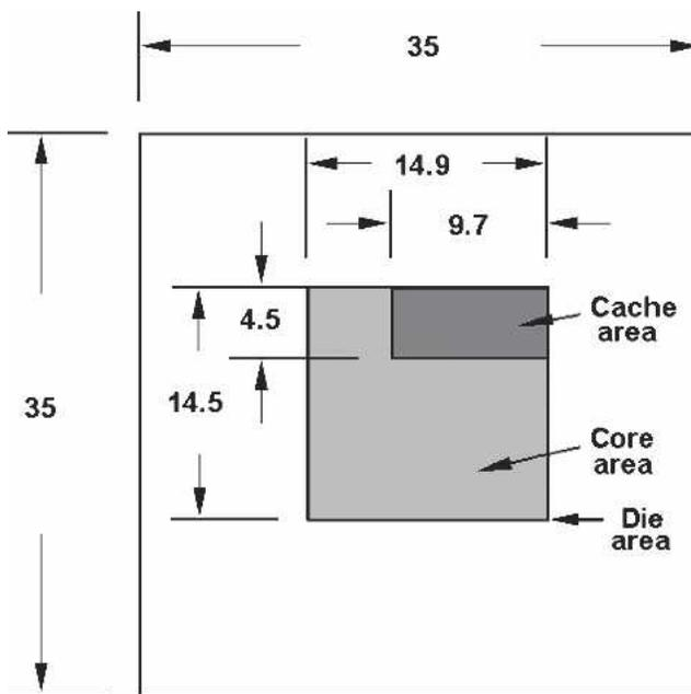
Fig. 4. Functional die layout for computer B. All dimensions are in millimeters and were taken from a photograph of the die.
