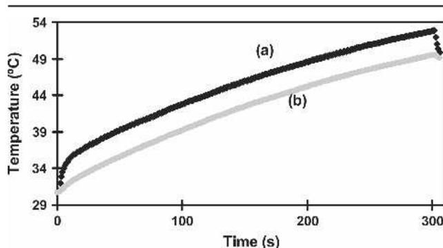
Fig. 7. Temperature versus time of computer operation (up to 5 min.) for computer B with carbon black paste as the thermal interface material: (a) microprocessor temperature and (b) heat sink temperature.
