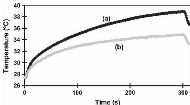
Fig. 6. Temperature versus time of computer operation (up to 5 min.) for computer A with carbon black paste as the thermal interface material: (a) microprocessor temperature and (b) heat sink temperature.
