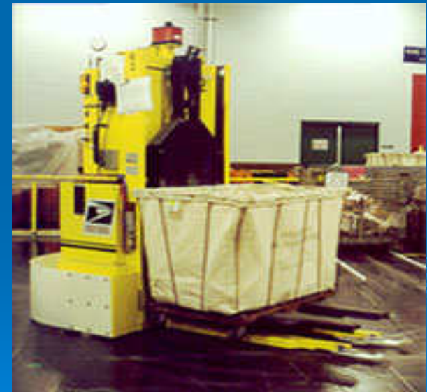
Load Capacity: 1,500 lbs Vehicle Type: Laser Guided Fork Lift AGV Products, Inc
