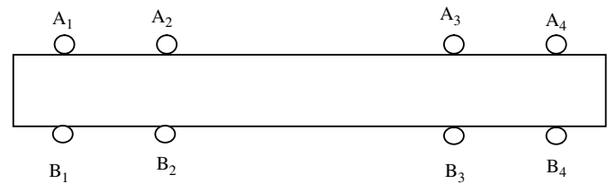
Fig. 1. Schematic of the edge of a composite to illustrate the concept behind the placement of electrical contacts. A_1 , A_2 , A_3 , A_4 are contacts on one surface; B_1 , B_2 , B_3 and B_4 are contacts on the opposite surface. All the contacts are strips of about 2 mm wide in the direction perpendicular to the length of the composite.
