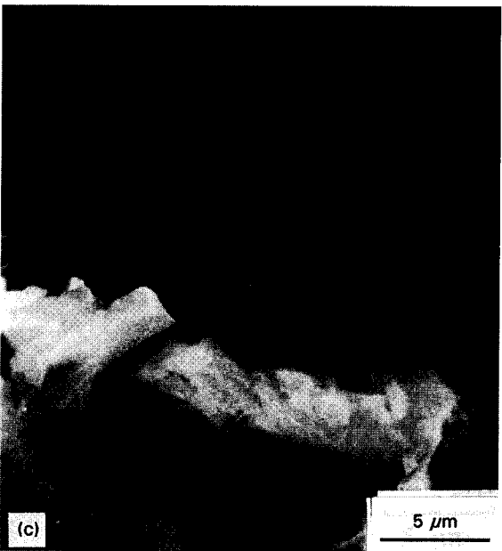
Figure 5 SEM photographs at various magnifications of composite B after heavy etching in 20% \text{NaOH} solution.
