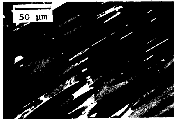
Figure 7 SEM photograph of the same composite as Fig. 6. No fibre breakage was observed.
